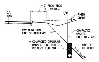
STORM, SEWER, OR UTILITY LINE PARALLEL TO ROAD OUTSIDE OF R/W
