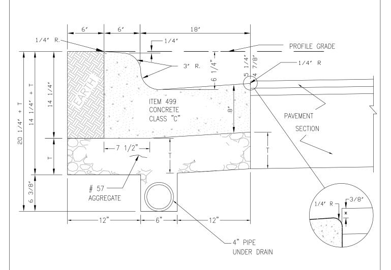
PAVEMENT SECTION THICKNESS -83/8" = T1.59 C.F. CONCRETE PER L.F.
