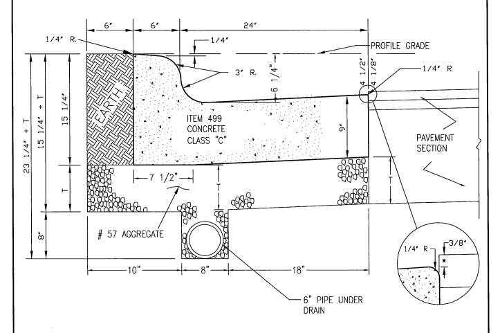
PAVEMENT SECTION THICKNESS -93/8" = T \* MAXIMUM GUTTER PAN CROSS SLOPE AT ALL HANDICAP RAMPS = 1.5%. TOP OF PAVEMENT MUST BE FLUSH TO GUTTER AT ALL HANDICAP RAMPS.
