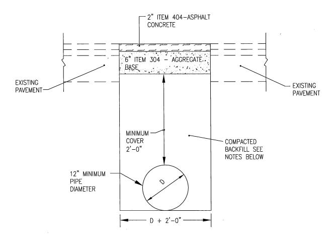
AGGREGATE BASE SHALL BE ELIMINATED WHEN CONTROLLED DENSITY FILL, ITEM 636, TYPE I OR II IS USED FOR COMPACTED BACKFILL.
