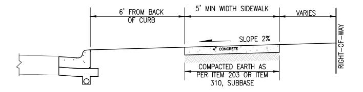
SIDEWALKS SHALL BE CONSTRUCTED WITH CLASS C CONCRETE (ITEM 499) WHICH SHALL CONTAIN 5% TO 8% ENTRAINED AIR AND A 3" MAXIMUM SLUMP. WHERE DRIVEWAYS CROSS THE SIDEWALK THE CONCRETE SHALL BE 6" THICK FOR RESIDENTIAL DRIVES, OR 8" THICK FOR COMMERCIAL DRIVES.
