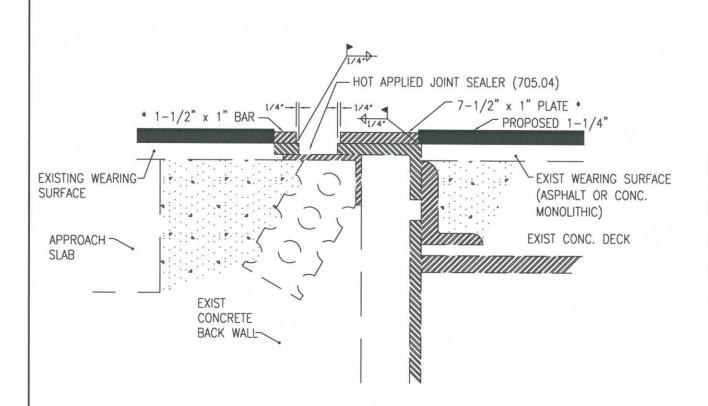
\* PLATE AND BAR HAVE BEEN SIZED BASED ON STANDARD STEEL EXPANSION JOINTS. CONTRACTOR SHALL VERIFY DIMENSIONS FOR EACH INSTALLATION. PLATE AND BAR SHALL BE 1/2" LESS IN WIDTH THAN THE EXISTING CONDITIONS.
