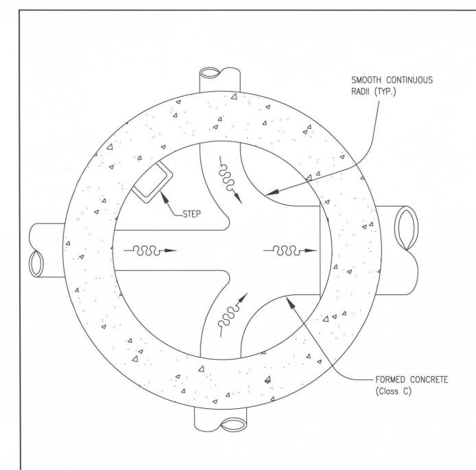
SECTION SHOWING METHOD OF TURNING SIDE DRAINS
