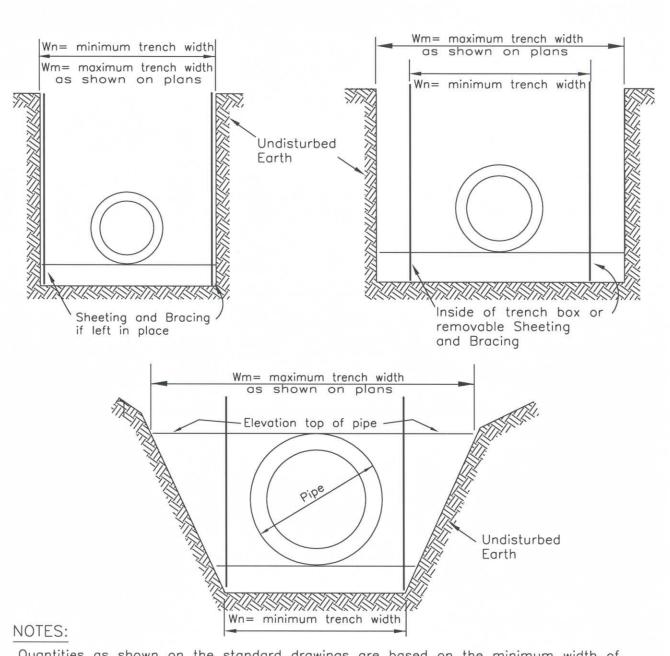
Quantities as shown on the standard drawings are based on the minimum width of trench (Wn). If an alternative trench is used the contractor will be required to extend the bedding, backing or encasement material across the entire excavated trench at the depth specified. The cost of the increased material shall be included in the price bid for Item 901.
