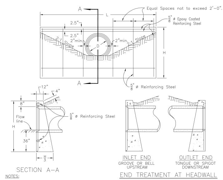
Headwall where required are for non-skewed culverts having a diameter or rise of 36" or less.
