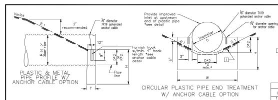
1 - Top Surface of 6" Inlet Headwall Extenssion
